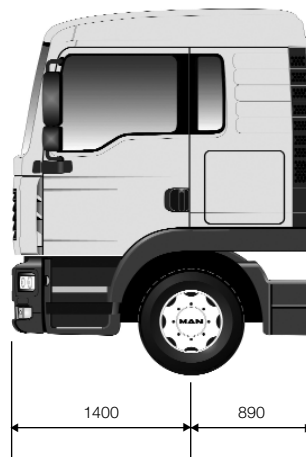
'L' Sleeper Additional Weight: 170 kg
