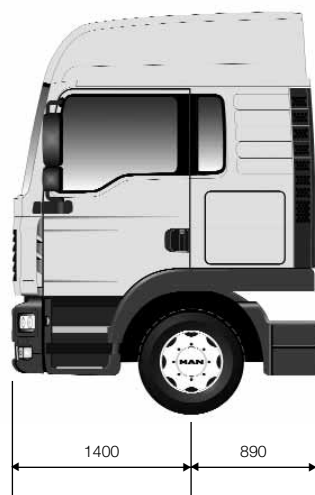
'LX' Sleeper Additional Weight: 235 kg
